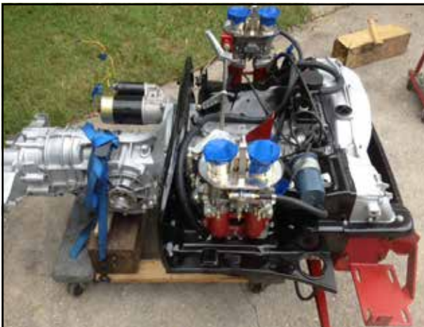
LEFT: Rebuilt drivetrain ready to install. With 96mm P/Cs, displacement was bumped to 2056.
